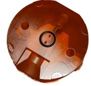
The volume of the measurement chamber above the electrode is 10  $\mu$ L ensuring the high resolution in the flow of the liquid.
