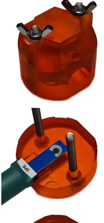
FlowCell chamber is designed for electrochemical measurements during the flow of the analyzed liquid. FlowCell is made by stereolithographic 3D printing from ABS resin.
